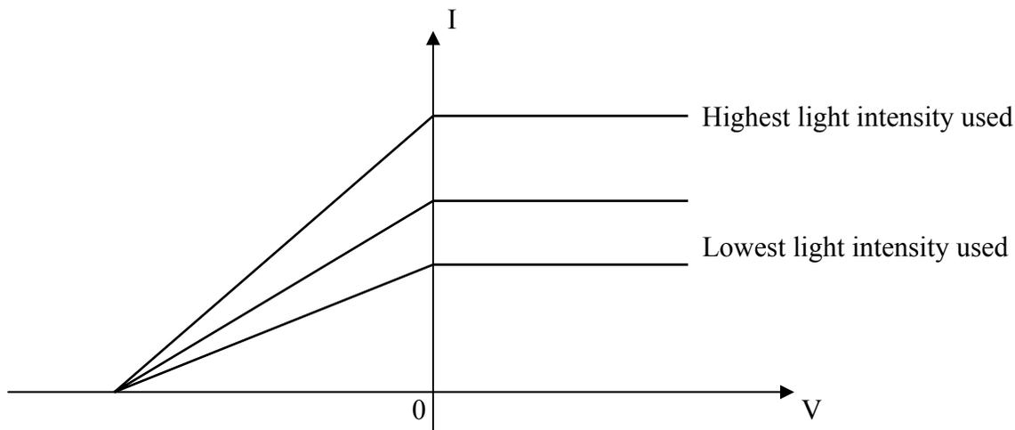
**Question 3** The photoelectric current remains constant when the accelerating voltage increases. Explain this finding using Planck's photon model.
