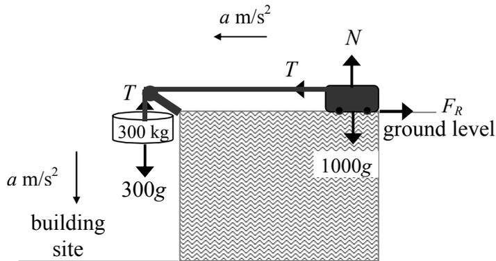
Resolving horizontal forces around the engine:
