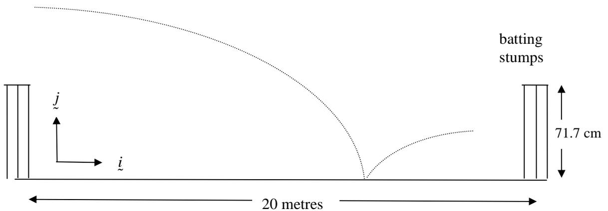
The horizontal ( easterly ) distance from the point where the ball leaves his hands to the stumps is 20 metres, and the cricket stumps are 71.7 cm high as shown in the diagram above.
