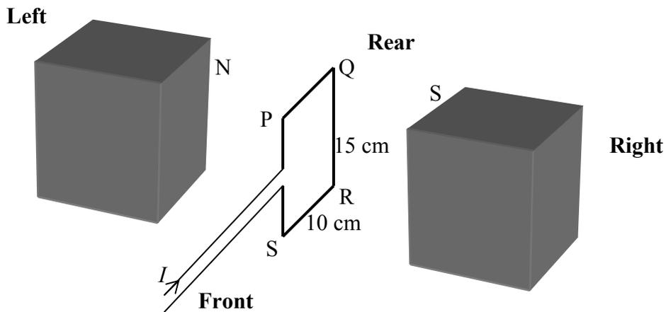
A rectangular loop PQRS (15 cm by 10 cm) of 20 turns of insulated copper wire is placed between two opposite magnetic poles as shown in the diagram above. It shows the initial orientation of the loop. There is an electric current  $I = 2.0 \text{ A}$  in the loop. The magnetic field is uniform  $B = 0.5 \text{ T}$  between the poles.
