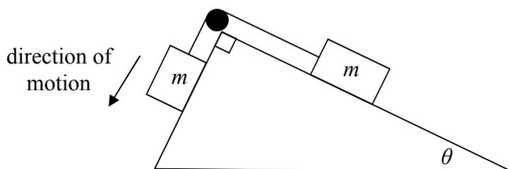
Two bodies each of mass,  $m$  kg, are connected on a back-to-back plane by a light string passing over a smooth pulley, as shown in the diagram. The coefficient of friction of the surface of each plane is  $\mu$ .
