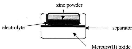
The diagram above shows the basic structure of a mercury-zinc button cell. The cell can be classified as an alkaline cell. The
