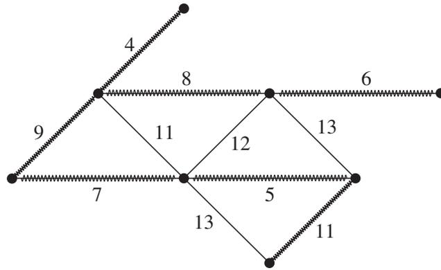
The edges selected in the above diagram are chosen by use of Prim's algorithm.
