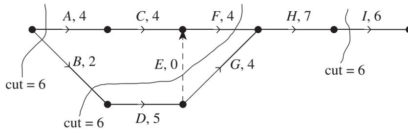
The ‘maximum flow’ is always equal to the ‘minimum cut’. The minimum cut is shown above. It happens to occur three times and is equal to 6 litres.
